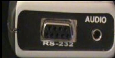
The PX has an Audio output jack for Amplified speaker or Recorder output.
